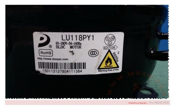
Pro.mbsm.pro, FUJIDENZO INVERTER, REFRIGERATOR, ISR-20SS, 532L, Compressor, Donper, inverter, LU118PY1, 1/3 Hp, HISENSE, 700 L, 108/to/250 W, variable speed, blcd, 5.8 cm3, R 600a, 75G, 65-180v, 54-140Hz
